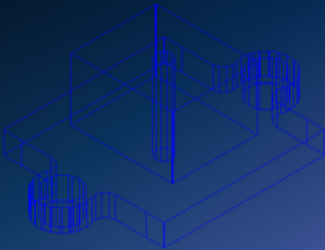
Cold finger for TEC and temperature sensor.
